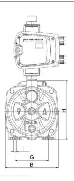
Height with controller fitted H2 + approx 246mm = 390mm
